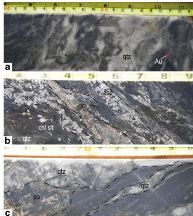
**Fig. 8** Images of representative sections of ore for the Golden pride Au deposit. **a** Silica ore showing the strong silicification of sericite-altered sandstone. **b** Chlorite ore showing arsenopyrite- and pyrrhotite-rich bands within chlorite-altered siltstone. **c** Chlorite ore showing a pyrrhotite-rich domain amongst strongly boudinaged and deformed quartz veins within chlorite-altered siltstone
